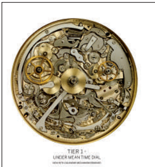
The Patek Philippe Henry Graves Supercomplication and its movement showing complications like perpetual calendar, chronograph and moonphase.
